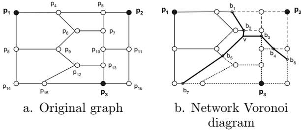
Figure 2: Example of a network Voronoi diagram (NVD)
