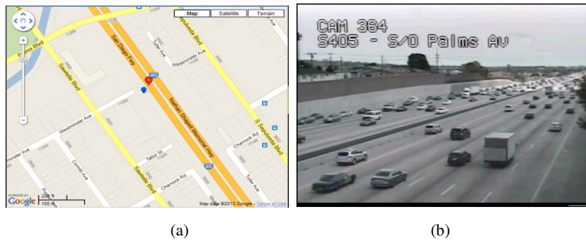
Fig. 7. Example of a good test case: (a) camera (blue dot) and loop detector sensor (red dot) are located very close, (b) good camera angle and low traffic condition
