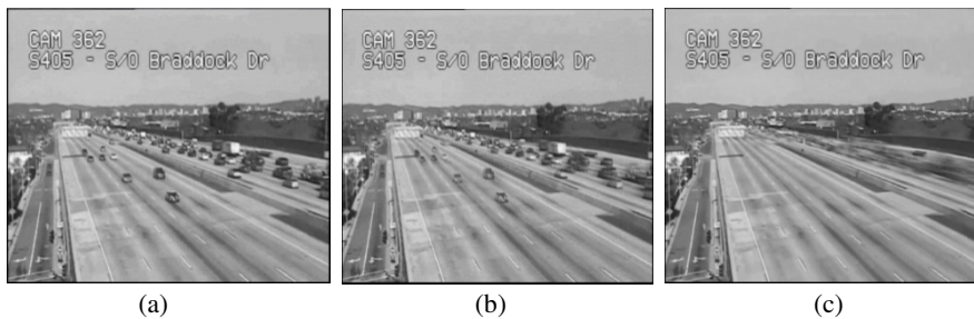
Fig. 3. Background extraction: (a) original background frame, (b) intermediate background, (c) final background
