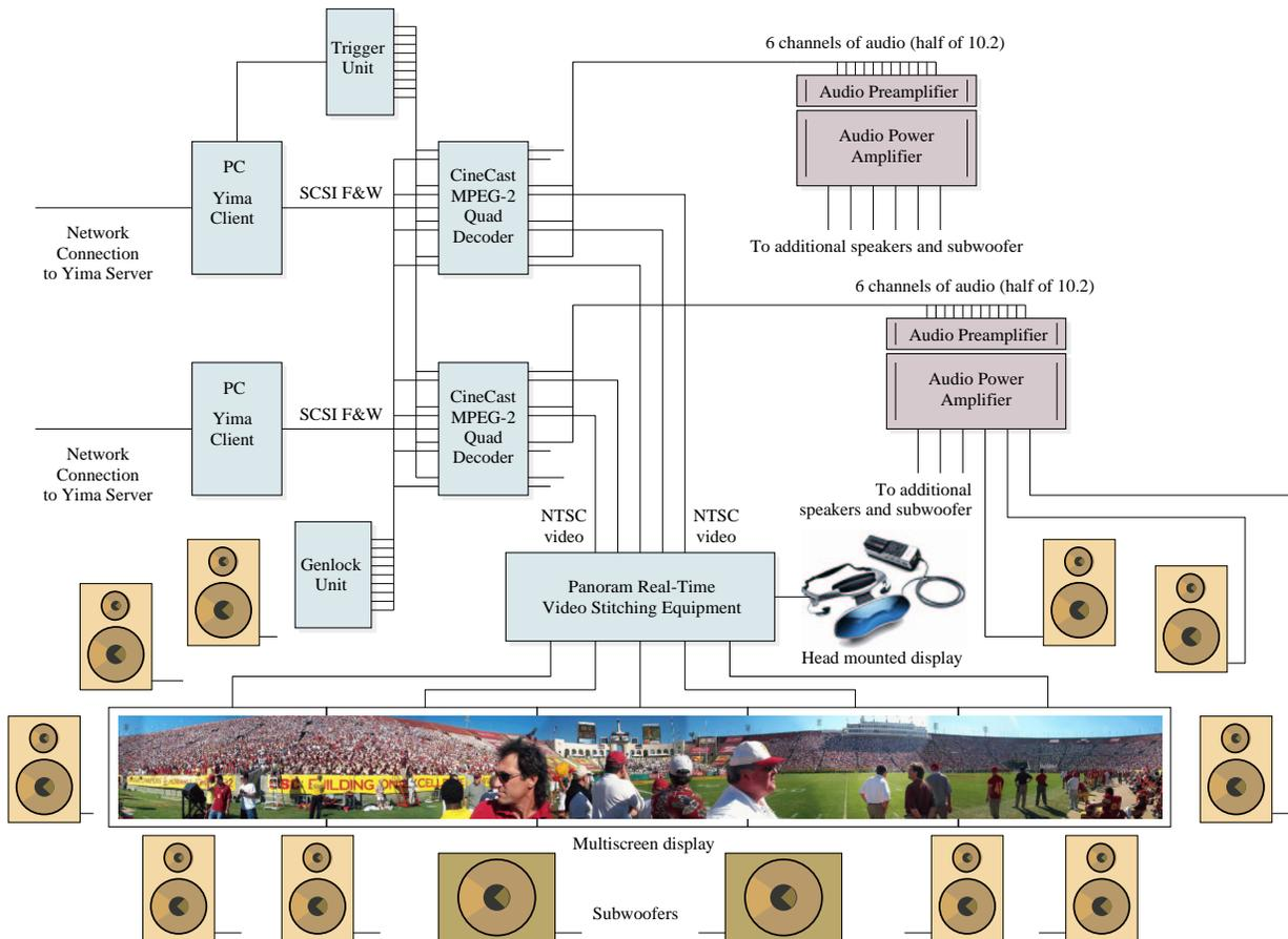
Figure 5: Panoramic video and 10.2 channel audio playback system block diagram. Two Yima clients are used to render 5 channels of synchronized video (i.e., a mosaic of  $3000 \times 480$  pixels) and 10.2 channels of synchronized audio (the 0.2 refers to two low-frequency channels, e.g., subwoofers).
