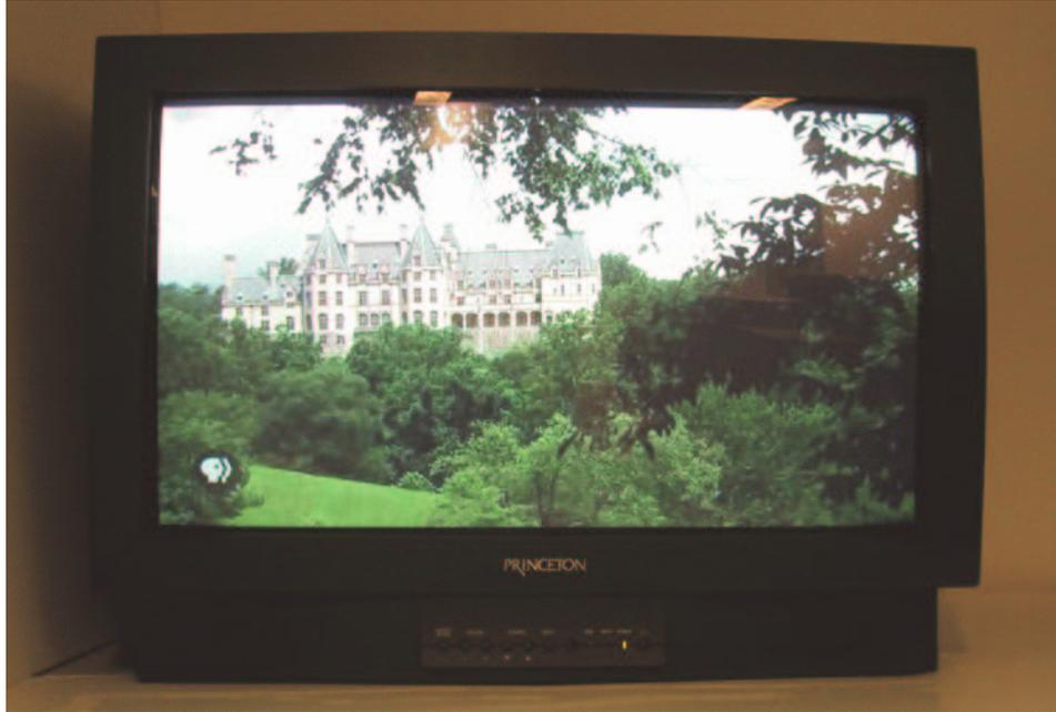
Figure 8: HDTV display connected to an Yima client. The Yima client can decode HD MPEG-2 formats in software up to the full the resolution of  $1920 \times 1080i$  (with some degradation in the frame rate on a 933 MHz PC). The picture shows a quarter-resolution video with  $960 \times 540p$  pixels compressed via MPEG-4.
