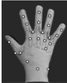
**Figure 1:** CyberGlove. Joint angles are measured at positions marked with a circle.
