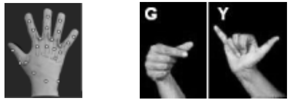
a. CyberGlove: Joint angles are measured at positions marked with a circle b. Some ASL signs are measured at positions marked with a circle
