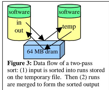
**Figure 3:** Data flow of a two-pass sort: (1) input is sorted into runs stored on the temporary file. Then (2) runs are merged to form the sorted output
