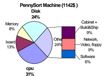
The key properties of this system are Intel Pentium II 266 MHz processor, Asus mother board, 64 MB of Synchronous 10 ns SDRAM, dual 3.5GB Fujitsu UltraDMA IDE drives, and NT Workstation, all for \$1,142. Given this price, the time allowed for a PennySort, computed by Table 2, is 828 seconds. The prices keep dropping. Today (the end of April 1998) <http://www.pricewatch.com/> reports that component prices have dropped 10% this month.
