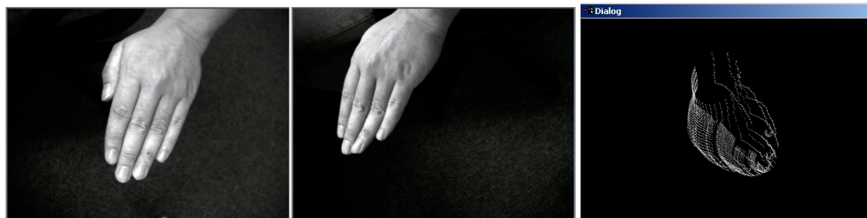
Figure 2. 3D shape of the inferred from the detected silhouettes without local edge analysis.
