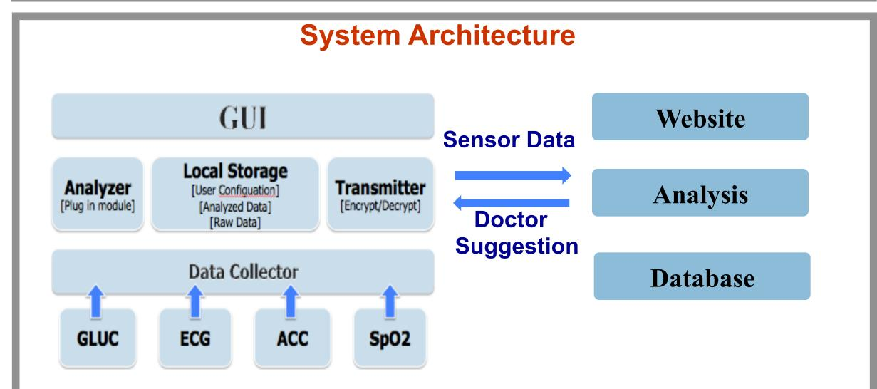
•Data collector aggregates different types of data into a single record. Local storage stores user configuration, analyzed data and raw data in the external storage.
