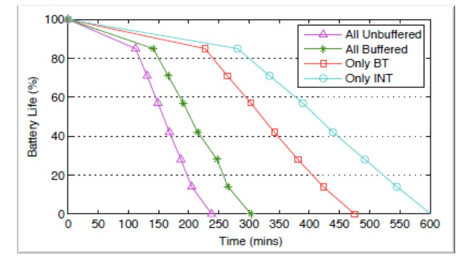
Dramatic battery drain reduces 200 hours standby to 5 hours. Even without external sensors the in-built sensors also drain battery.
